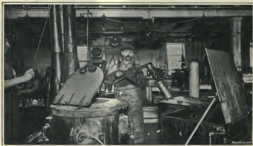
Fig. 9. Heat-treating Shrapnel Shells, using a Hoskins Electric Barium-chloride Bath Furnace
